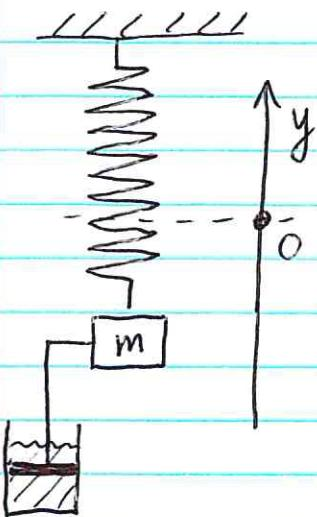
$$ma = F_{\text{spring}} + F_{\text{damping}} + F_{\text{gravity}}$$
