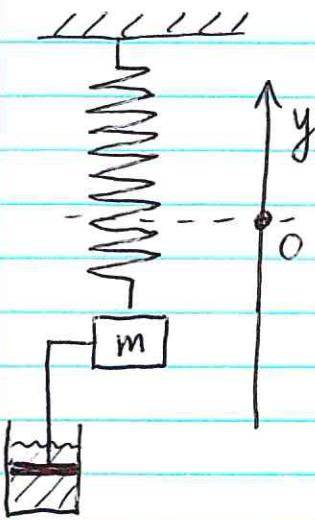
$$ma = F_{\text{spring}} + F_{\text{damping}} + F_{\text{gravity}}$$
