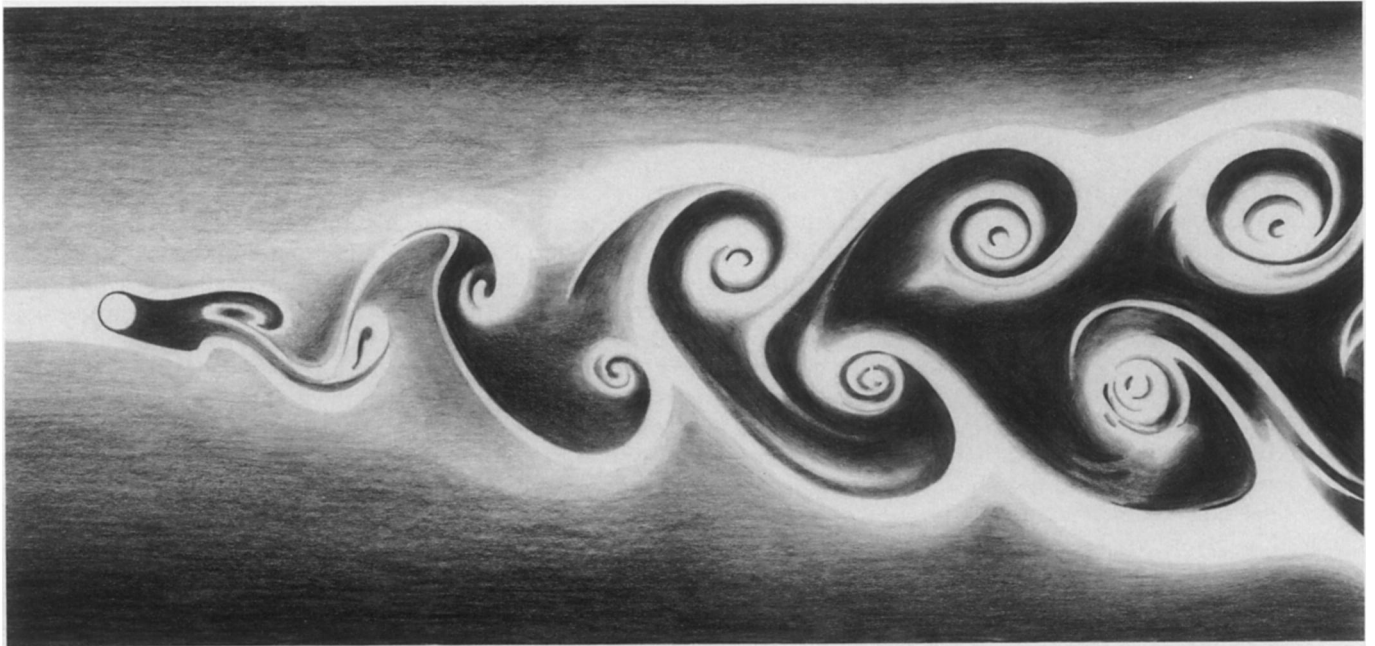
Figure 2. Kármán vortex street, a pattern of alternating vortices created by the confrontation of a nonstreamlined body and an airstream and initially suggested as the source of the periodic impulses that drove the Tacoma Narrows Bridge to collapse.
