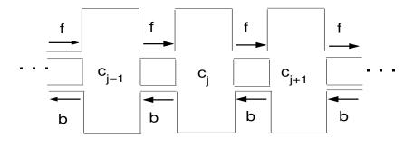
Each element  $\Delta x$  is modeled as a tank connected to its "neighbors" by two pipes, as schematically shown above. The rates of the flows to the right and to the left are maintained at values f and b, respectively. Your derivation should follow that of Eq. (17), where you may assume A = 1 for simplicity.
