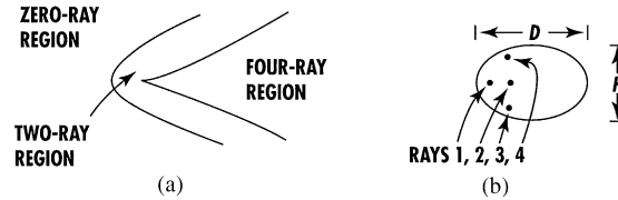
Fig. 25. (a) The partitioning of angular regions according to the hyperbolic–umbilic diffraction catastrophe, arising in connection with rainbow scattering from spheroidal drops (see [224,230] for details). (b) The rays in the horizontal plane (1,2) and the skew rays (3,4) contribute to the generalization of the rainbow for scattering from spheroidal drops. (Redrawn from [224].)
