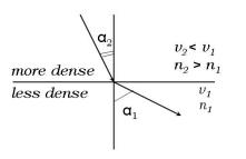
$$\frac{\sin \alpha_1}{v_1} = \frac{\sin \alpha_2}{v_2} \tag{1.1}$$
