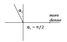
Side note: If light falls from an optically more dense medium into optically less dense one (e.g., from water into air, with  $n_{\text{water}} > n_{\text{air}}$ ), then total internal refraction will occur when  $\alpha_2 > (\alpha_2)_{\text{crit}}$ . Here  $(\alpha_2)_{\text{crit}}$  is calculated by setting  $\alpha_1 = \pi/2$  (see the figure on the left). Then from (1.2) we have (verify):
