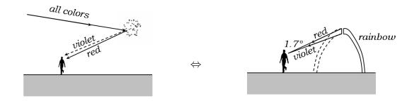
The two figures above illustrate the following. The red ray coming from a given drop ("drop A") goes lower than the violet ray coming from the same drop. If the violet ray from drop A enters observer's eye, then the red ray from the same drop hits below the eye. Equivalently, the red ray must come from a drop that is *higher* then drop A to enter observer's eye. This is why red color is seen above the violet color in a primary rainbow.
