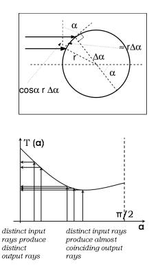
The number of rays coming out of the droplet in the angular sector  $\Delta T$  is, similarly:  $N_{\text{out}} = \rho_{\text{out}} \cdot r \Delta T \cdot \cos \alpha$ , where we have used the fact that the rays come out at the same angle  $\alpha$  to the normal radius at which they came in: see the figure at the end of this page. Setting  $N_{\text{out}} = N_{\text{in}}$ , as explained above, one finds:
